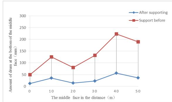
Figure 4. Before and after the central bottom support displacement diagram
