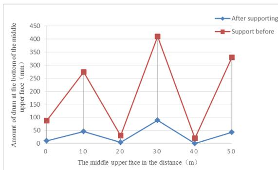
Figure 3. In the middle upper floor support before and after the displacement map
