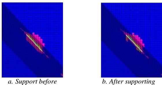
Figure 2. Working face floor support before and after the distribution of plastic zone
