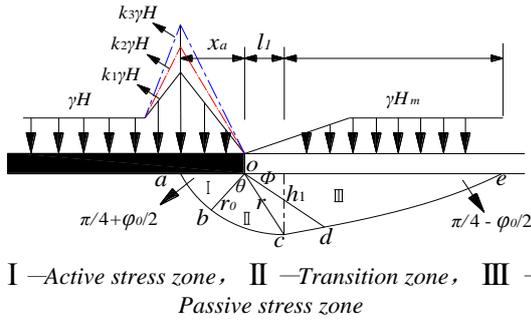
Figure 1. Along the Steep Face Towards the Bottom Plastic Failure Zone Profile Model Diagram
