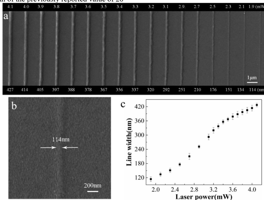
**Fig. 3** (a) SEM images of fabricated lines at a constant writing speed of  $10 \mu\text{m s}^{-1}$  with the laser power ranging from 1.9 mW to 4.1 mW. (b) Magnified SEM image of the line of 114 nm at the power of 1.9 mW. (c) Laser power-line width relationship of (a).
