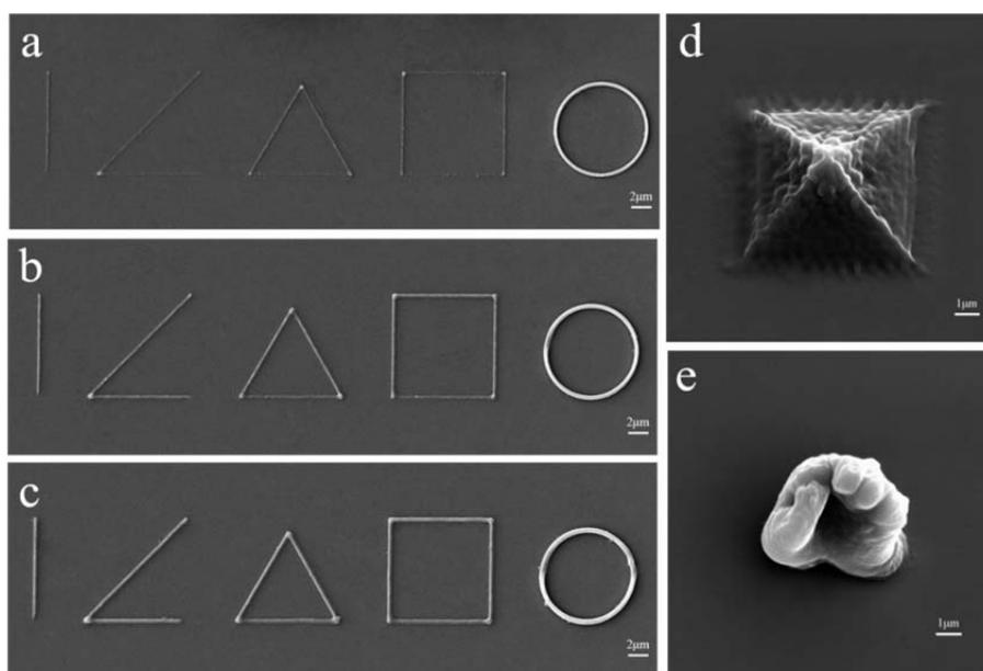
**Fig. 4** (a-c) Fabrication geometry at a constant writing speed of  $10 \mu\text{m s}^{-1}$  and the laser power are 3 mW, 4 mW and 5 mW, respectively. (d) The pyramid structure was fabricated with laser power of 3 mW and a scanning speed of  $10 \mu\text{m s}^{-1}$ . (e) The pyramid structure was fabricated with laser power of 5 mW and a scanning speed of  $10 \mu\text{m s}^{-1}$ .
