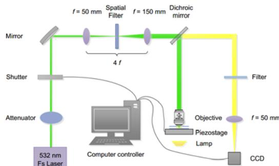
**Fig. 1** schematic of experimental setup for TPP microfabrication.
