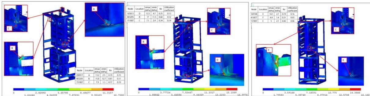
Fig. 6 Stress Nephogram of Electrical Cabinet under Fatigue Strength Working Condition from 1 to 3
