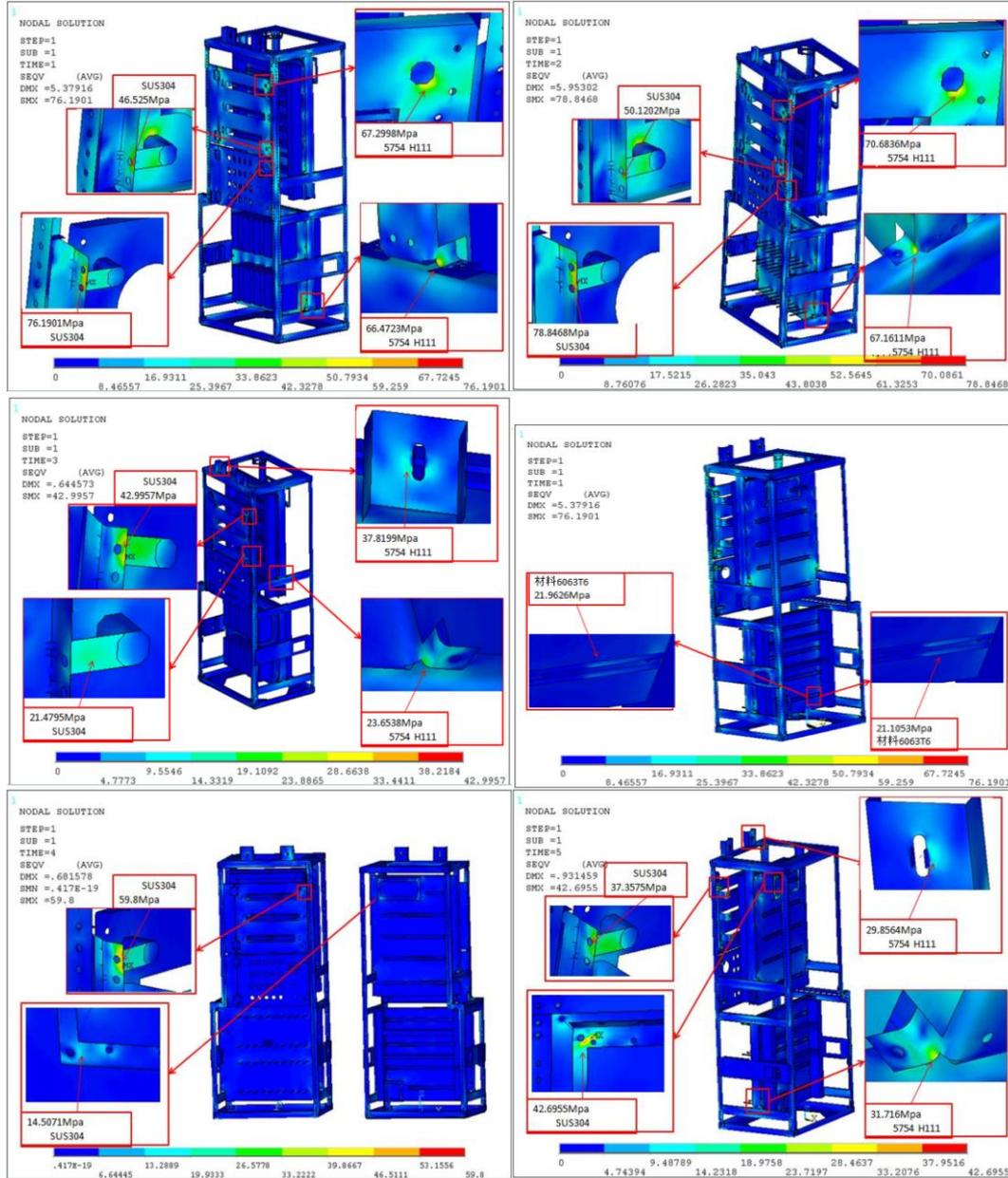
Fig. 5 Stress Nephogram of Electrical Cabinet under Static Strength Working Condition from 1 to 5
