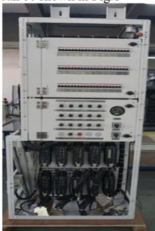
Fig. 1 Driver's Cab Electrical Cabinet
