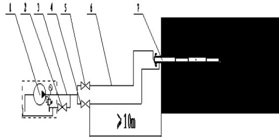
1- High pressure water injection pump; 2- Regulating valve of return water; 3,6- High pressure hose; 4,5-Inlet valve; 7- Two-segmented hole sealer
