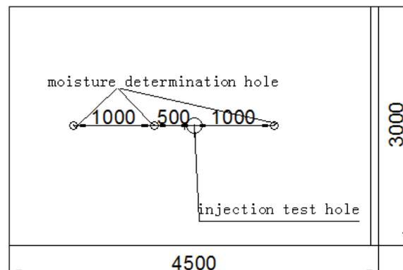
Figure 4. Layout of water injection test hole and moisture determination hole
