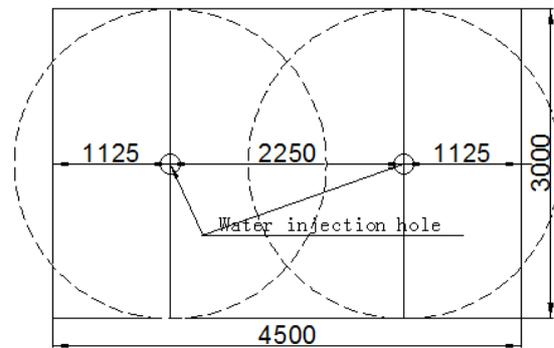
Figure 5. Layout of water injection holes in working face
